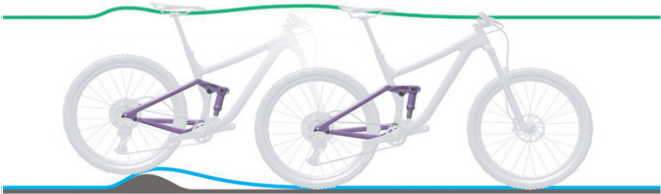
Figure 218: Excessively hard damping in the rear frame damper on bumps
