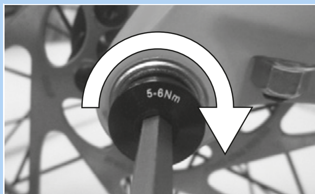
Figure 46: Tightening the securing screw
