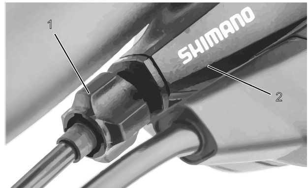
Figure 128: Adjusting sleeve (1) for the single-cable, Bowden-cable-operated gear shift with shifter housing (2), example
