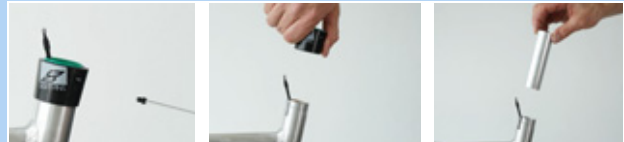
Figure 176: Removing the outer sleeve and slide bushing
