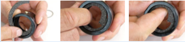
Figure 147: Inserting the felt ring
