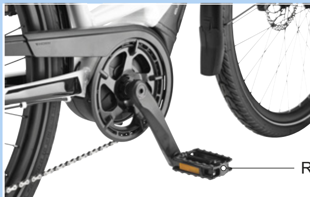
Figure 59: R-pedal in the right-hand crank arm
