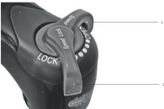
Figure 201: Changing compression adjuster to a harder setting
