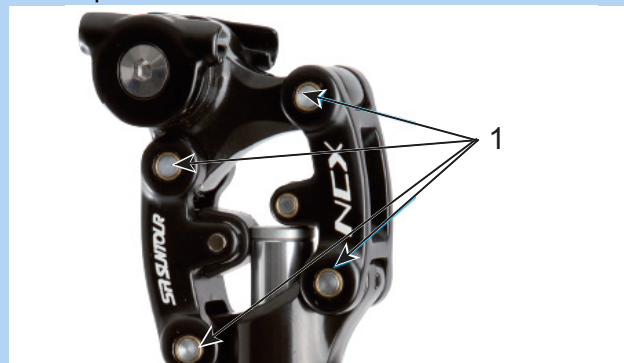
Figure 133: SR Suntour suspension seat post lubrication points
