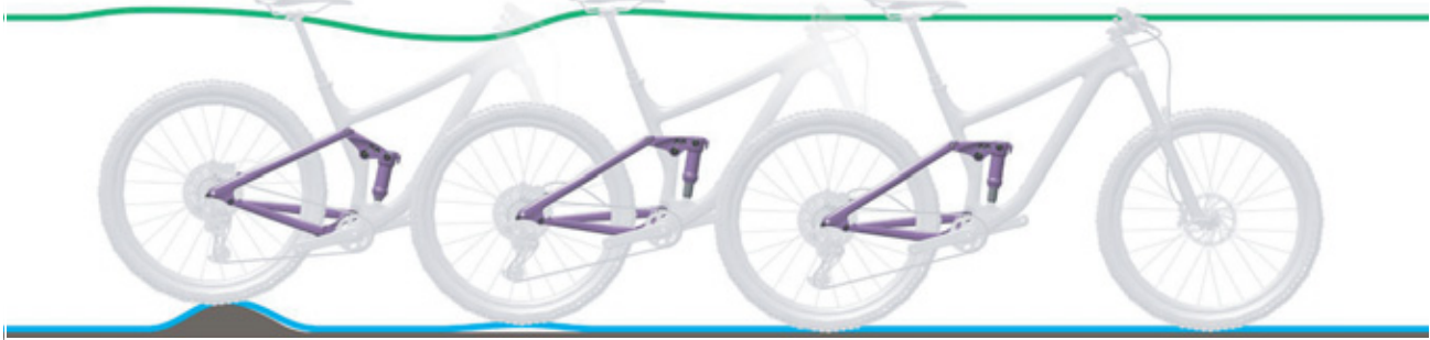
Figure 212: Rear frame damper rebounding too quickly
