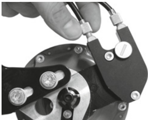
Figure 127: The tension adjuster on Rohloff hub versions with external switch control is located on the cable box positioned on the left-hand side
