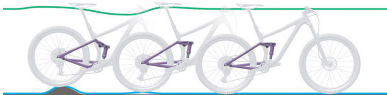
Figure 220: Rear frame damper rebounding too quickly
