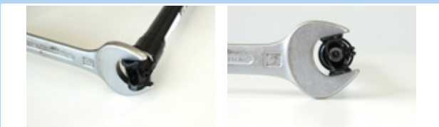
Figure 155: Securing against twisting
