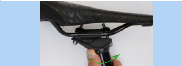
Figure 185: Opening the height adjustment
