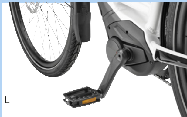
Figure 58: L-pedal in the left-hand crank arm
