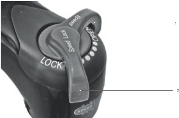
Figure 203: Changing compression adjuster to a softer setting
