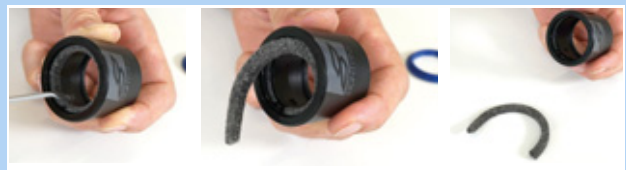
Figure 145: Removing the felt ring
