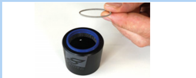
Figure 178: Removed spring washer
