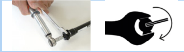
Figure 156: Setting in a clockwise direction
