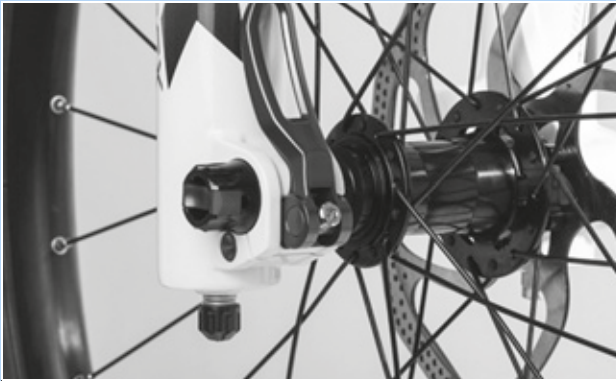
Figure 131: Adjusting the quick release clamping force
