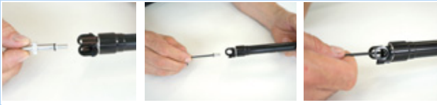
Figure 153: Fastening the cartridge valve lid
