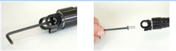
Figure 154: Unscrewing the valve cap
