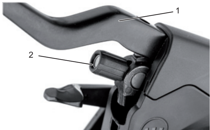
Figure 55: Brake lever (1) of the hydraulically operated rim brake with setting bolt (2)
