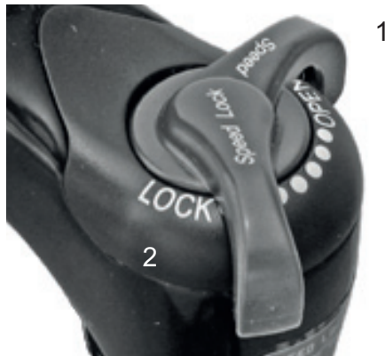
Figure 46: Suntour compression adjuster with the OPEN (1) and LOCK (2) positions
