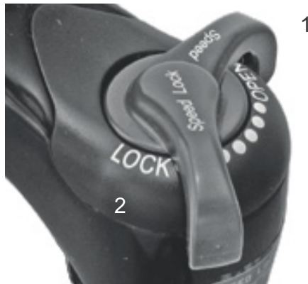
Figure 55: Suntour compression adjuster with the OPEN (1) and LOCK (2) positions
