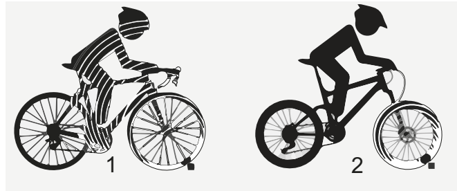
Figure 5: Bicycle without suspension (1) and with suspension (2) when riding over an obstacle
