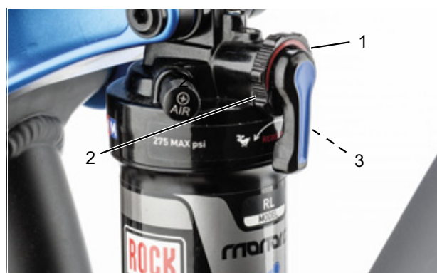
Figure 82: Setting the rebound damper strength on the rear frame damper setting wheel (1)
