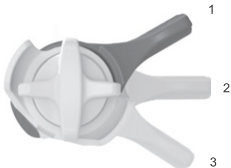
Figure 77: FOX compression adjuster on the rear frame damper with the OPEN (1), MEDIUM (2) and HARD (3) positions
